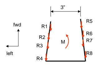
Shear load at rivets: R1=R2= ... = R8 = 1050/3/4 = 88 lbs
